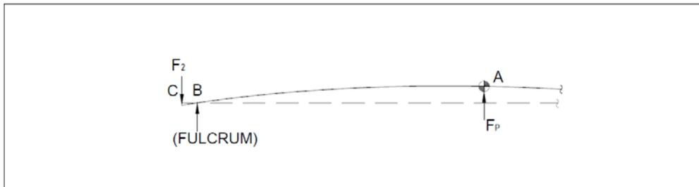
Diagram 5. Manhole Riser with Lip Bar Free-body diagram of highlighting pullout force,  $F_p$
