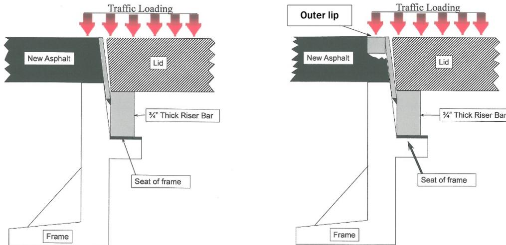
Diagram 1. Profile of AHP Type 1 (left) versus that of bar welded on top of riser assembly
