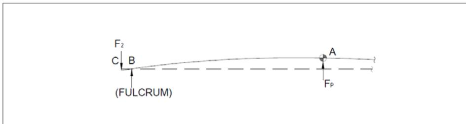
Diagram 3. AHP Type 1 Riser Free-body diagram of riser highlighting pullout force,  $F_p$
