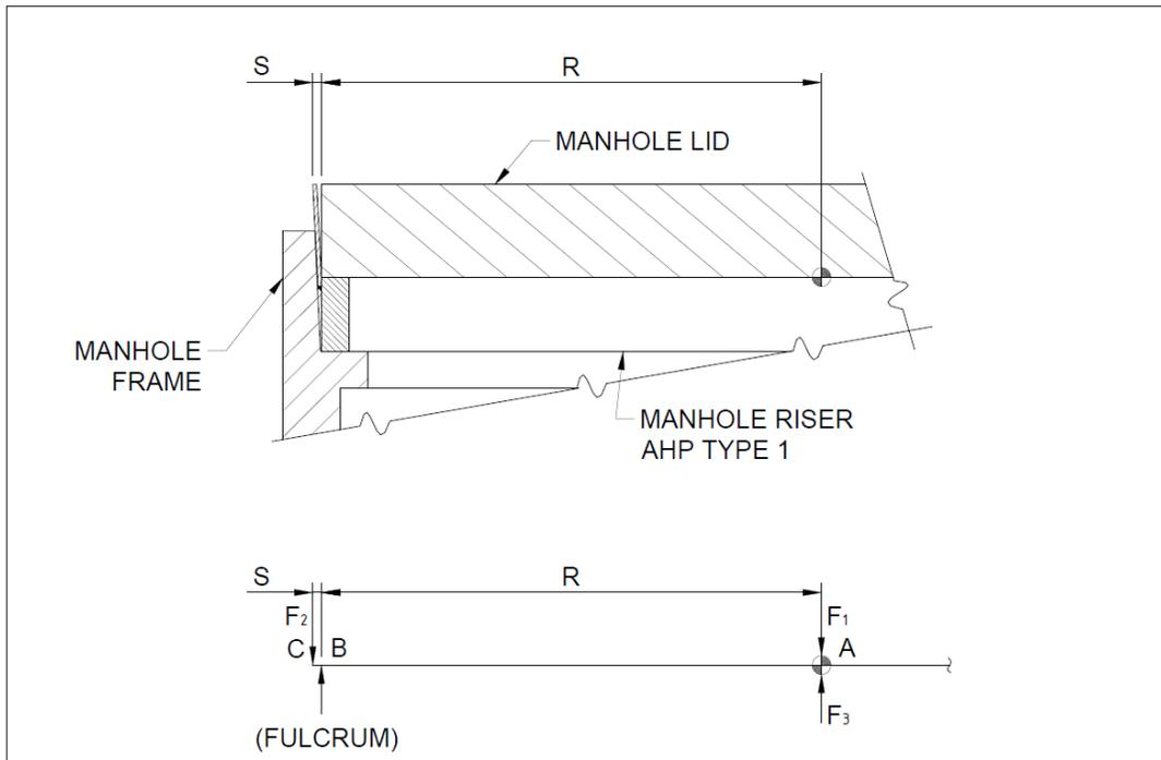
Diagram 2. AHP Type 1 Expandable Riser Example: Riser assembly in manhole frame (above), Free-body diagram of riser assembly (below)
