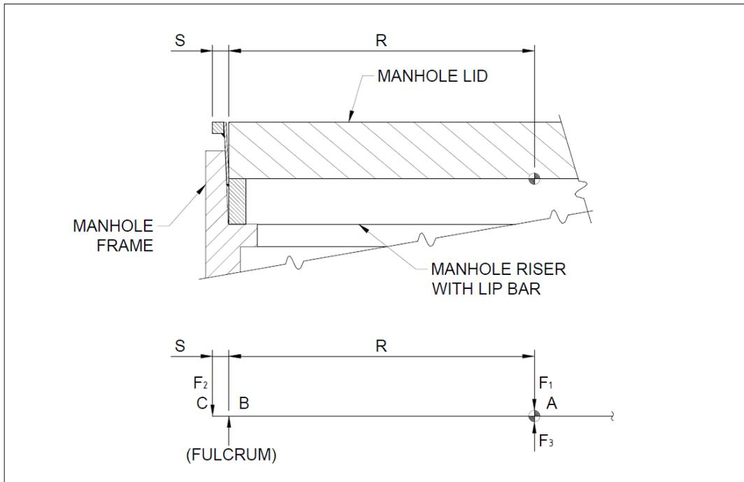
Diagram 4. Manhole Riser with Lip Bar Example: Riser assembly in manhole frame (above), Free-body diagram of riser assembly (below)
