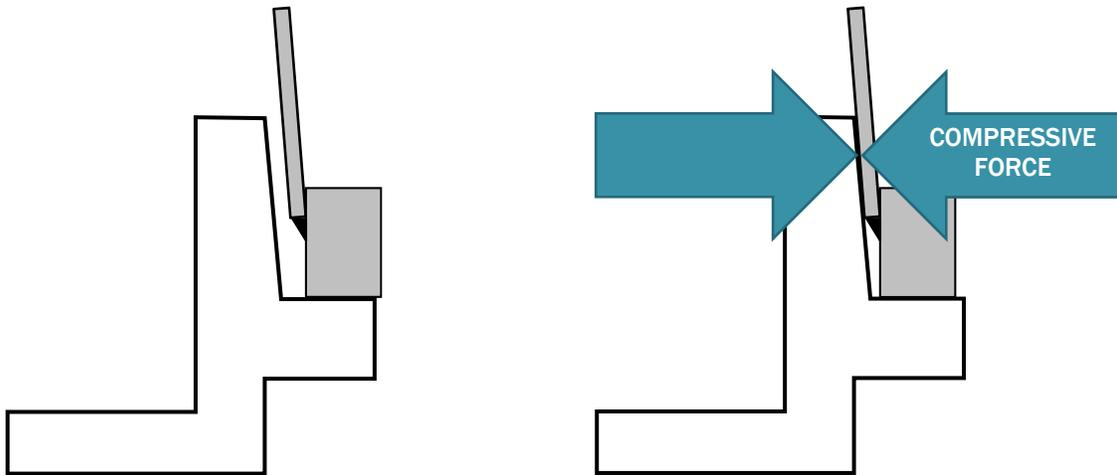
*Diagram 6. Riser prior to expansion (left) and riser after expanded into frame (right)*
